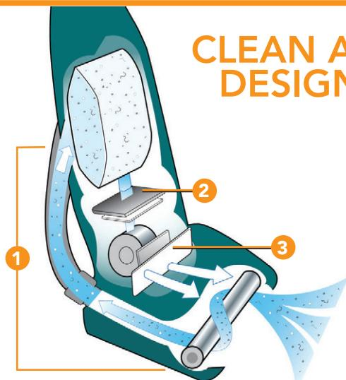
1. Dirt is pulled in and drawn through the vacuum bag.
